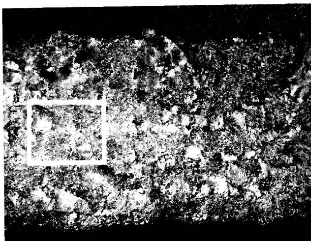
FIG. 7.—Etched surface of a mat-gold specimen of good compaction ( \times 25 ). The dendritic structure of the crystalline mat gold is broken down during compaction so that the condensed specimens are composed chiefly of broken crystal fibers. The gold is highly reflective in areas of condenser impact and the void spaces appear dark.
