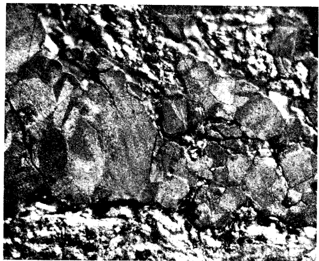
FIG. 10.—An uncondensed mat-gold specimen ( \times 375 ) is a mass of small crystallites that have dendritic structure.
