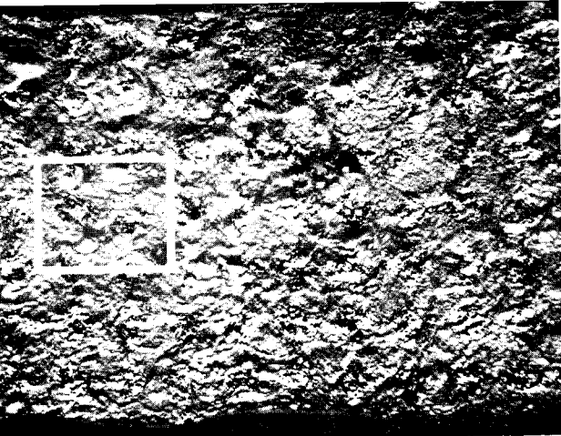
FIG. 1.—Etched surface of a gold-foil specimen of good compaction ( \times 32 ). Underneath the polished surface the dense gold appears light and the void spaces dark when exposed by etching.
