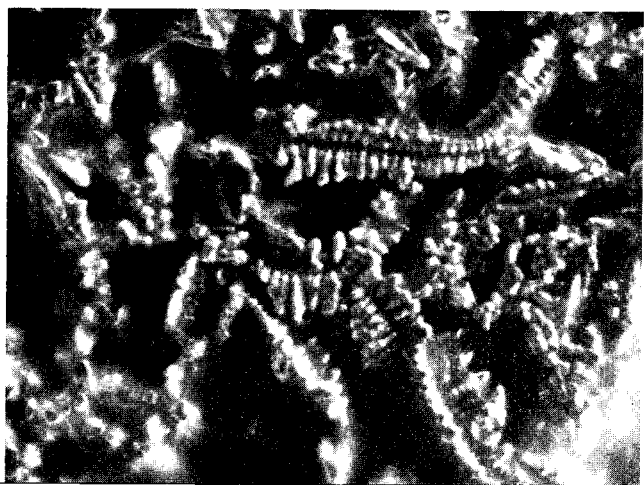
FIG. 10.—An uncondensed mat-gold specimen ( \times 375 ) is a mass of small crystallites that have dendritic structure.
